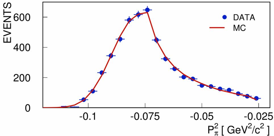
Kinematic parameter  $P_{\pi^0}^2$  - longitudinal momentum squared of kaon in a rest frame where longitudinal momentum of  $\pi^+\pi^-$  is zero under  $K_L \rightarrow \pi^+\pi^-\pi^0$  hypothesis
