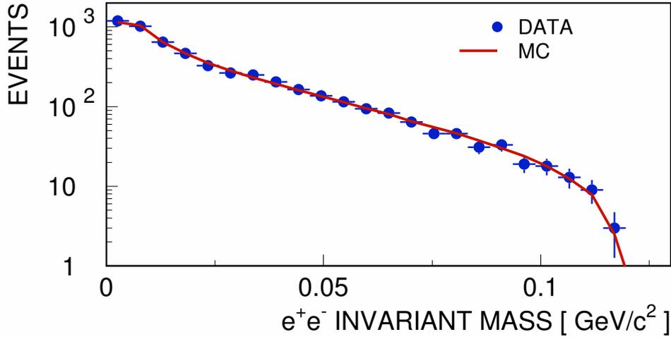
$e^+e^-$  invariant mass for DATA and Monte Carlo events. The events are required to have  $M_{ee} \geq 2 \text{ MeV}/c^2$  to suppress  $K_L \rightarrow \pi^+\pi^-\gamma$  decays with external conversions
