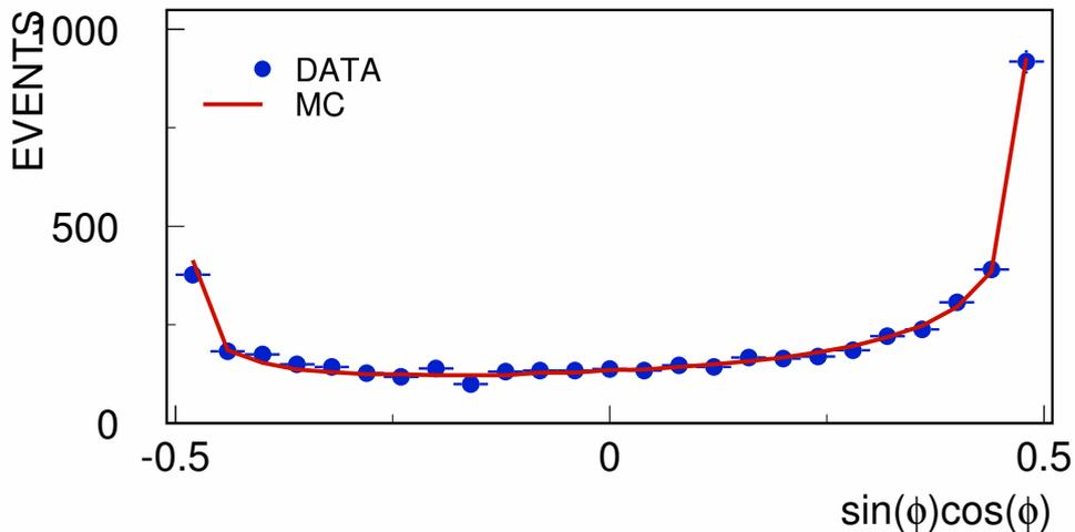
Parameter  $\sin\phi\cos\phi$  for an angle between  $\pi^+\pi^-$  and  $e^+e^-$  planes for DATA and Monte Carlo events
