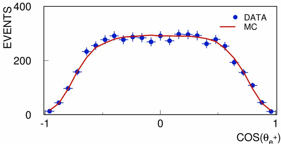
Angle between  $e^+$  and  $\pi^+\pi^-$  system in  $e^+e^-$  rest frame for DATA and Monte Carlo events
