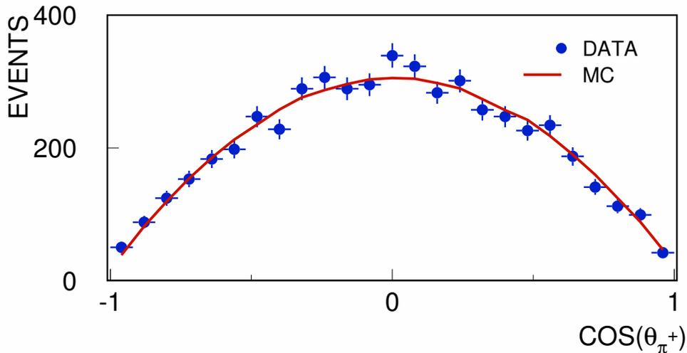
Angle between  $\pi^+$  and  $e^+e^-$  system in  $\pi^+\pi^-$  rest frame for DATA and Monte Carlo events
