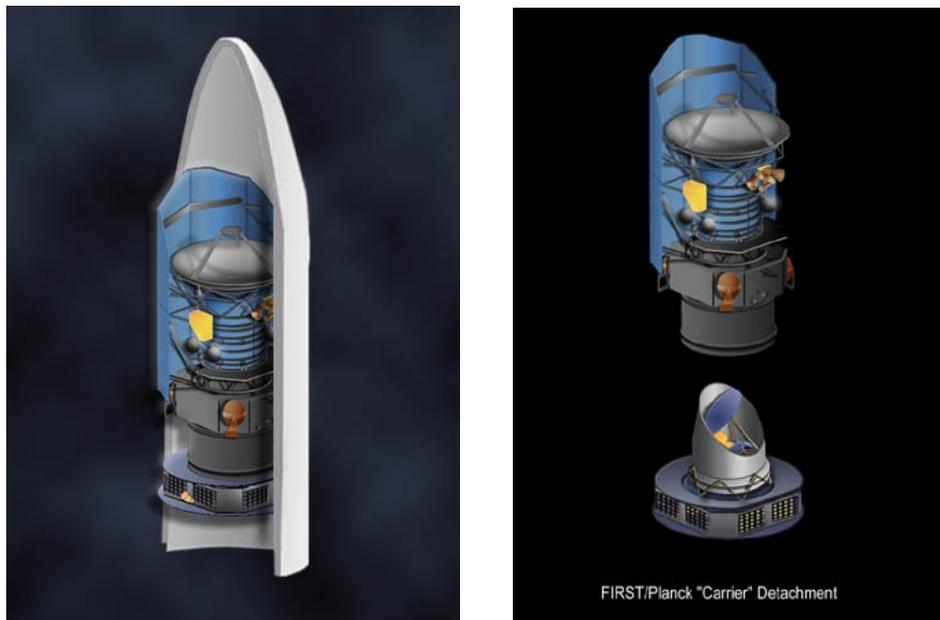
Figure 1: Common assembly of FIRST and PLANCK in the Ariane 5 launcher.
