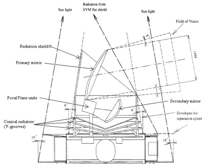
Figure 3: The new architecture of the PLANCK payload.
