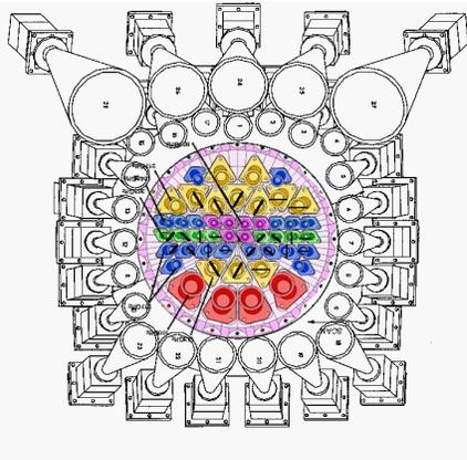
Figure 2: Face-on view of the PLANCK focal plane, HFI (inner) and LFI (outer).
