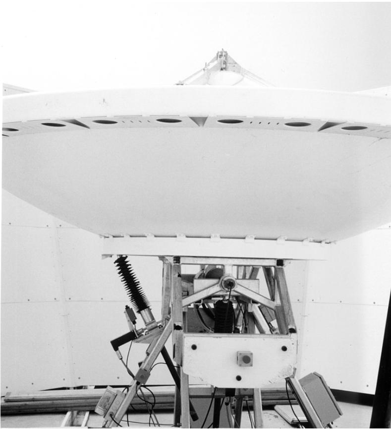
Figure 2: One of the two 3.7 m dishes that comprise the single baseline source monitoring system for the VSA (M. Jones). Each dish is housed in its own enclosure to prevent ground-spill. These enclosures are located just to the south of the VSA main array enclosure at the Observatorio del Teide, Tenerife.
