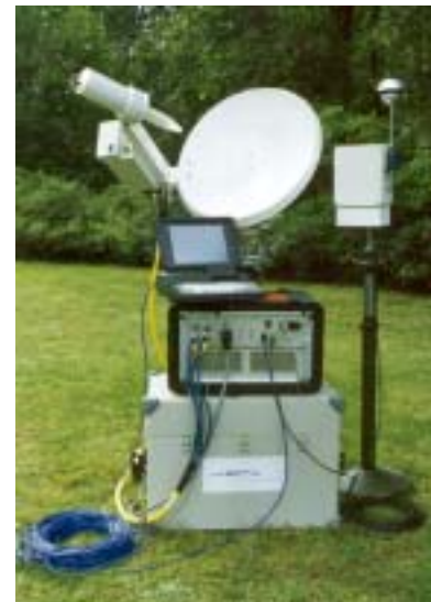
Typical MWL ground terminal
