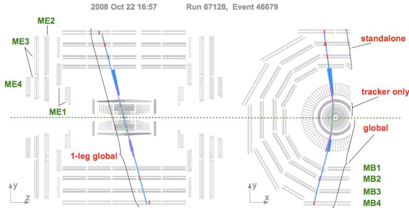
Figure 2: Event display of a cosmic muon crossing CMS.
