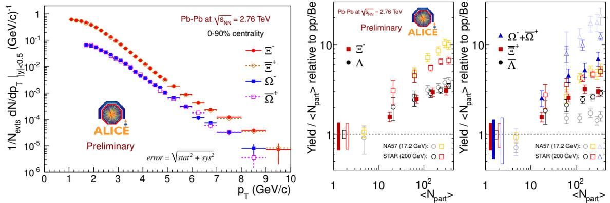
Figure 2: Transverse momentum spectra for  $\Xi^-$ ,  $\Xi^+$ ,  $\Omega^-$  and  $\bar{\Omega}^+$  in the 0-90% centrality range, on the left. On the right: enhancement for hyperon yields measured at mid-rapidity and for different centralities by ALICE (filled points), compared with SPS and RHIC data (open points). The vertical bars indicate the quadratic sum of statistical and systematic error. ALICE’s measurement of the  $\Lambda$  enhancement is not reported, as still in progress.
