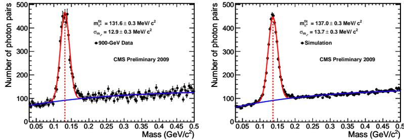
Figure 2: Photon-pair invariant-mass distribution ( $|\eta| < 1$ ) in data (left) and Monte Carlo (right). Also shown is a fit of the  $\pi^0$  mass peak by a Gaussian (red line). The fit mean value and resolution are  $131.6 \pm 0.3$  and  $12.9 \pm 0.3$   $\text{MeV}/c^2$  respectively for the data and  $137.0 \pm 0.3$  and  $13.7 \pm 0.3$   $\text{MeV}/c^2$  for the simulation. The combinatorial background is fit by an exponential function (blue line).
